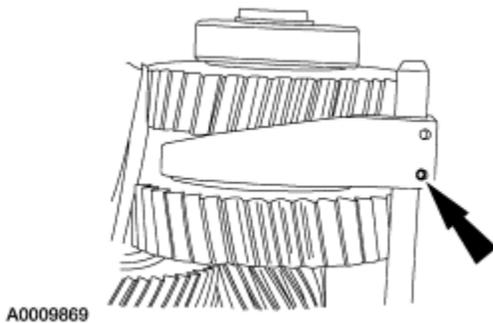
20. Remove the low/reverse gear shift fork and shift rail.
