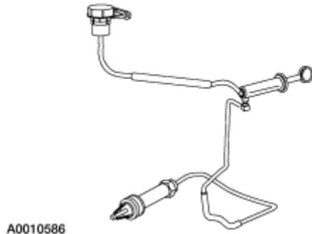
10. Correctly route the clutch hydraulic tube and attach the clutch hydraulic reservoir to the wiring tray.
