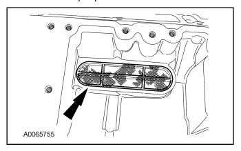
2. If the oil cooler was not replaced, install a new gasket in the oil cooler assembly cover.
