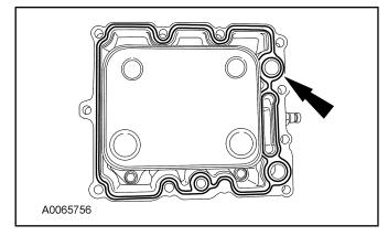
NOTICE: In the event of a catastrophic engine failure, always install a new oil cooler. Foreign material cannot be removed from the oil cooler.
